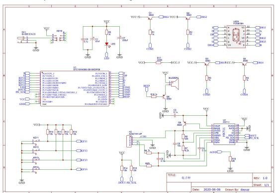
Working principle: STC15W408S single-chip microcomputer is used as the main control, weighing dedicated AD
